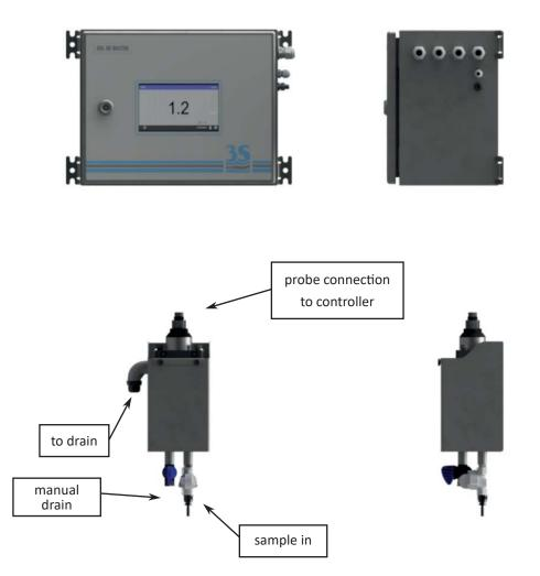
The sample reservoir (cod. A46U10035) should be mounted preferably under the controller. The sample line must be connected to the inlet below the container, optionally a flow sensor can be installed on the same line to detect the presence of the sample.
