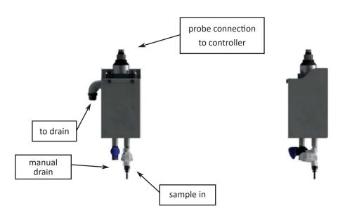
The sample reservoir (cod. A46U10035) should be mounted preferably under the controller. The sample line must be connected to the inlet below the container, optionally a flow sensor can be installed on the same line to detect the presence of the sample.
